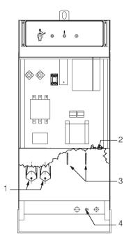
Connect a suitable welding and return cable to the contacts (3) marked \( \frac{1}{1} \) on the front of the power source.
